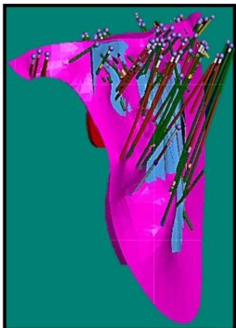
3D model of showing the proposed shape and relationship of Dyke 2, 3, 5, 6, 7, and 8 with previous intersecting drill holes
