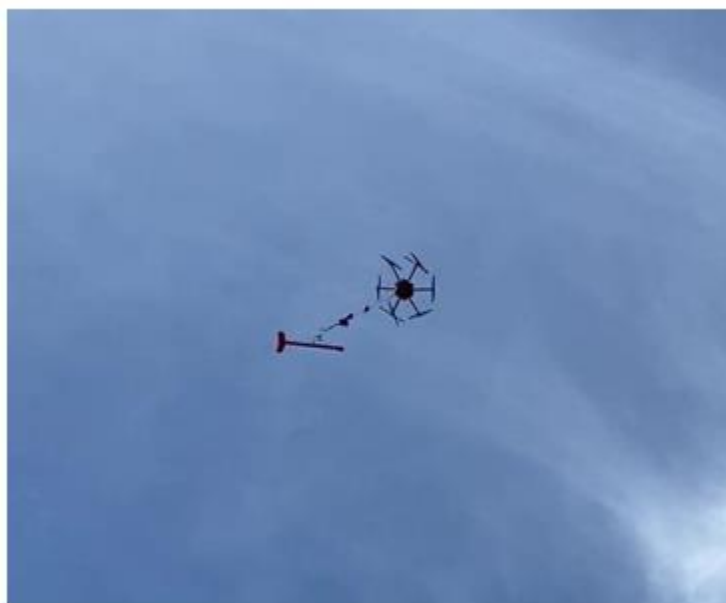
Figure 1. A magnetometer towed by a UAV or drone measuring the magnetic signature of the rocks on the ground over the Zoro Lithium Property.
