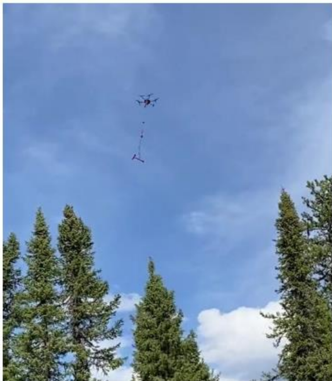
Figure 2. A magnetometer towed by a UAV or drone measuring the magnetic signature of the rocks on the ground over the Zoro Lithium Property.
