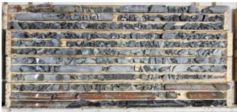
Figure 4 - A further pegmatite was intersected below the fault between 84.4 and 86.65 meters on Dyke 8
